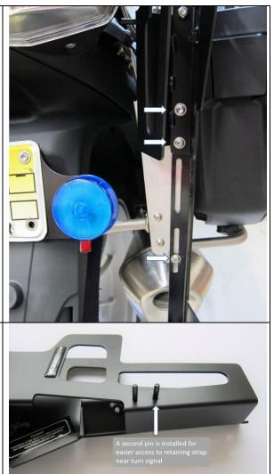
Later production rifle mounts are drilled and tapped for an M5 x .8 threaded pin to provide a more convenient pin location for the retaining strap – included with Long Rifle mounting bracket orders.
