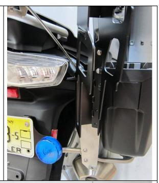
Per the example above, position the lower leg so that the distance from the inside of the muzzle cup to the center of the charging handle slot is 26". You may need to trim the length of the lower leg slightly if you are using a shorter barrel length.
