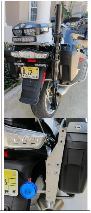
Secure the upper assault rifle mount to the upper two holes in the bracket using the M6 x 16 Torx bolts, securing with M6 nylock nuts. Snug but don't tighten fully yet.
